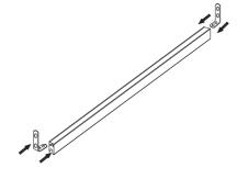
Insert the locking brackets (E) into the top cover (G) and fix it with screws (F). Attention: The concave side must face downwards.
